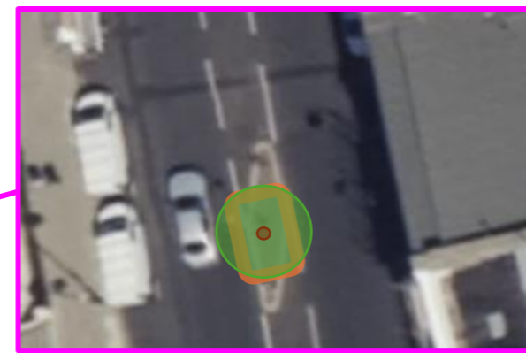
Tree pit 1 (TP1) – Replace existing island with 2.5m island and tree pit
